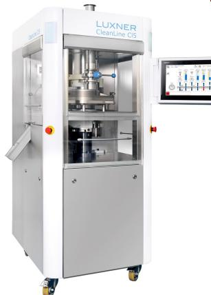
Our intuitive software (developed and programmed by Luxner) offers, among other things, password log, error log, event log, recipe management, automatic versioning of the recipes, batch log, press force control, single sorting and network connection.
